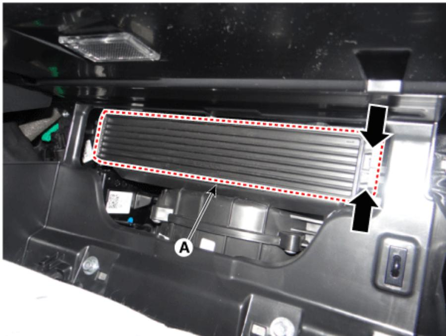
4. Replace the air filter (A) with a new one according to the direction of air filter.
