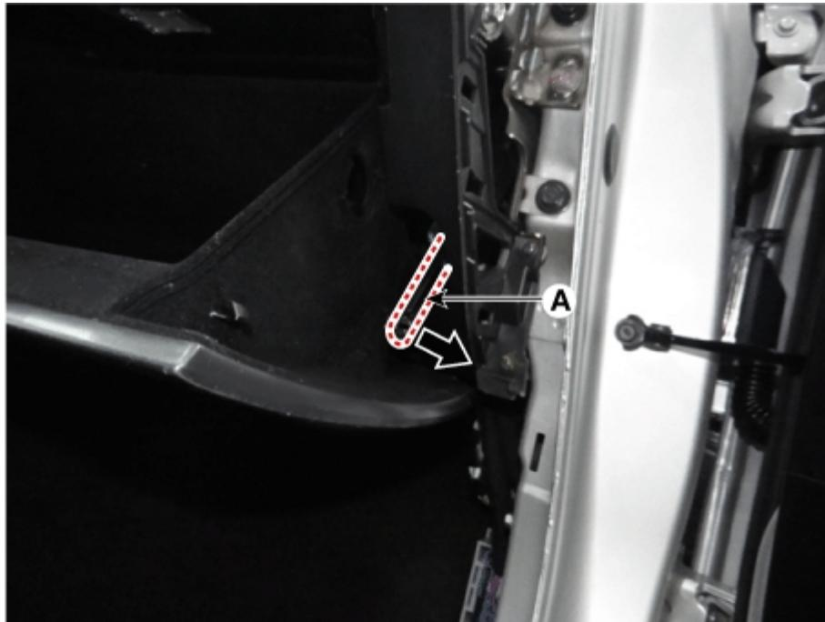
3. Remove the filter cover (A) by pressing the knob.
